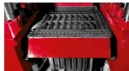
Multi-cavity mould for sand-lime bricks
