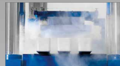
Pressing of salt blocks with mould spraying
